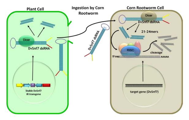
Figure I-1. Diagram of MON 87411 dsRNA Oral Delivery to Suppress DvSnf7 Expression via the RNAi Pathway in CRW
